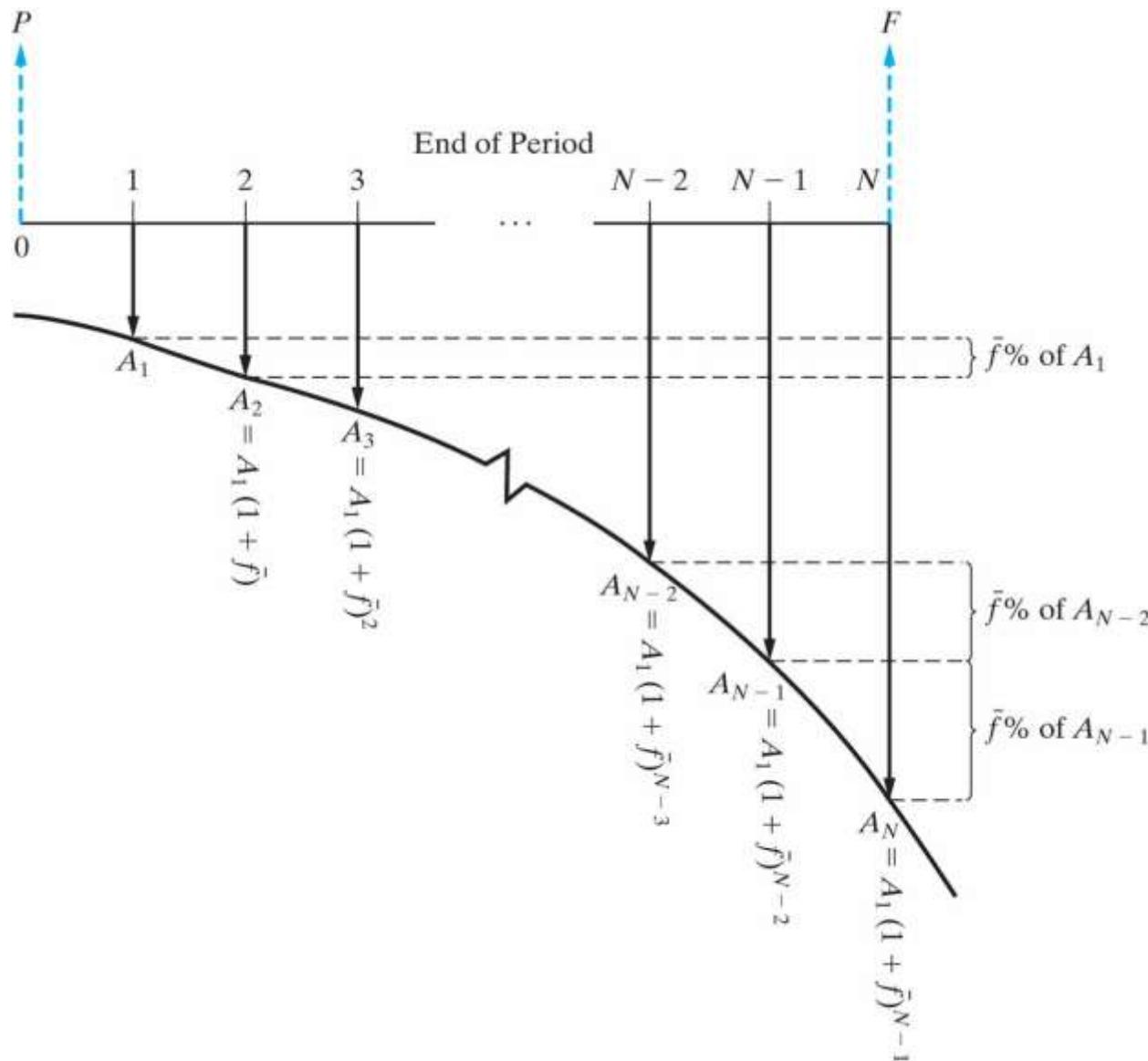
We can find the present value of a geometric series by using the appropriate formula below.
