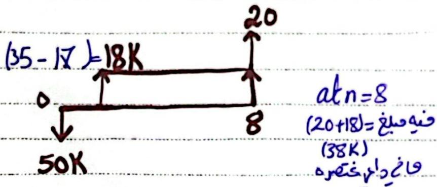
$$\rightarrow F_0 = -50K \quad | \quad F_1 = 18K \quad | \quad F_8 = 18K + 20K = 38K$$
